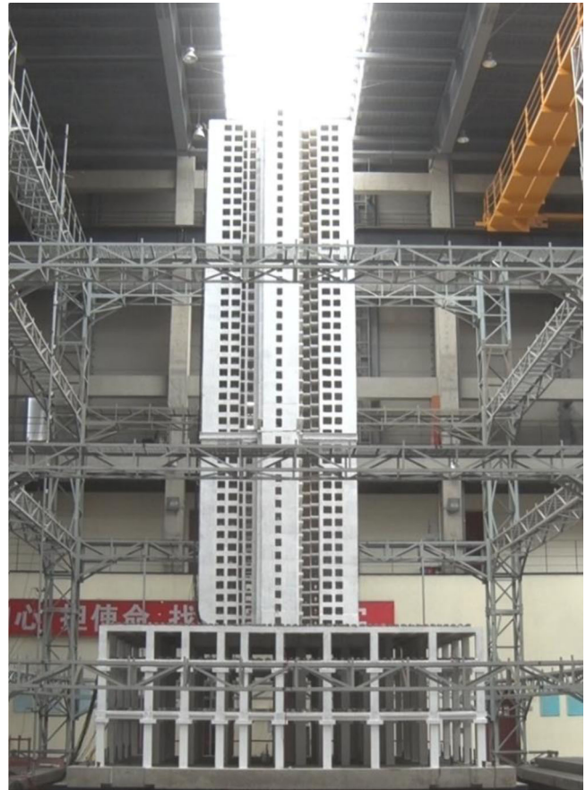
FIGURE 14 Shaking table test model
